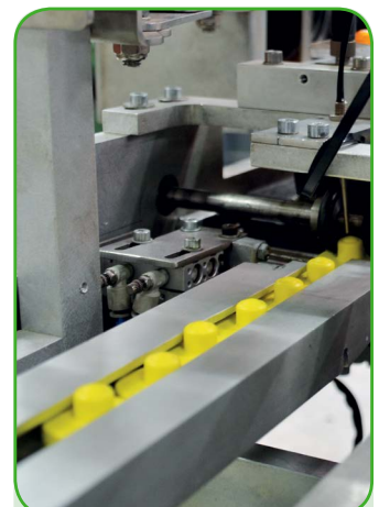
Programming and printing of electronic transponders
